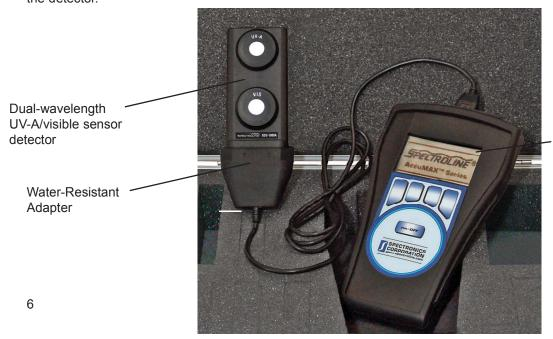
LCD window with numbers, units, modes and system status. Displays multiplexed data from UV-A/visible output.
