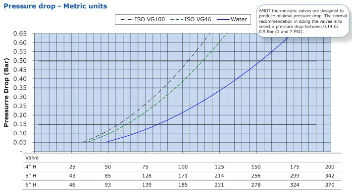
Flow Rate for Water (m<sup>3</sup>/hr)
