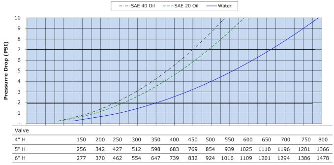
Flow Rate for Water (US gpm)
