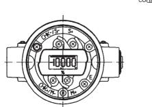
Terminal connection diaphragm (Terminal screw size: M4)
