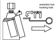
Extract the clip putting the extraction tool (KM/3062) in the hole of the security clip then pull hard to extract the clip.
