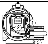
Connect the ground wire to the ground connecting screw (2).
