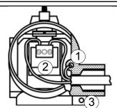
Connect the ground wire to the ground connecting screw (2).
