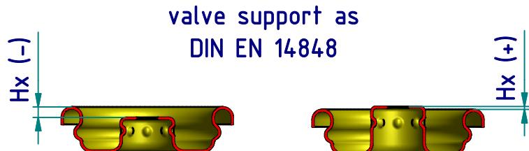
the measurement can be in progress at the valve support and on the complete can.
