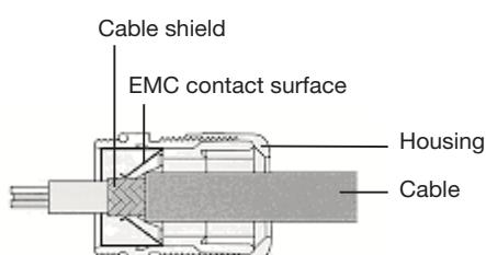
Fig. 7-1: EMC screw connection
