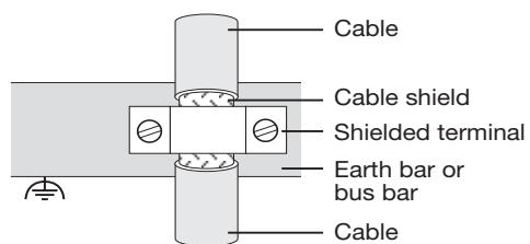
Fig. 7-2: Earthing the cable shield (example)
