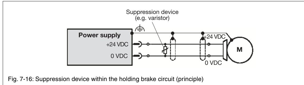
Fig. 7-16: Suppression device within the holding brake circuit (principle)
