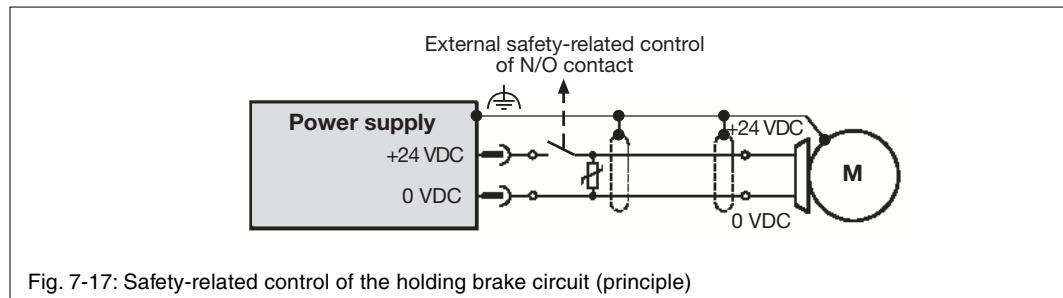
Fig. 7-17: Safety-related control of the holding brake circuit (principle)
