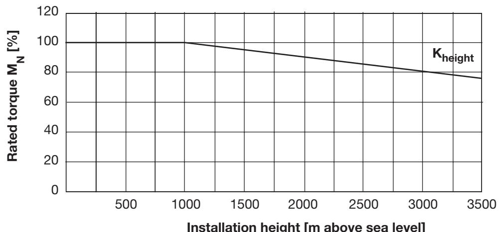
Fig. 12-1: Permitted torque in relation to installation height
