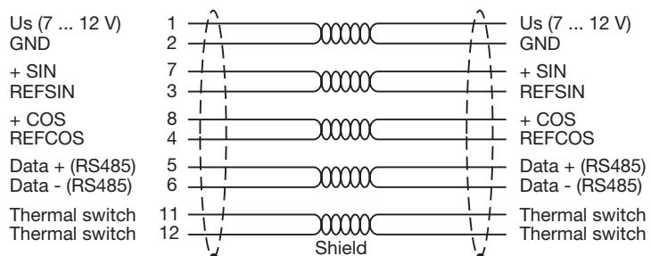
Fig. 7-6: Connection cable for Hiperface rotary encoder
