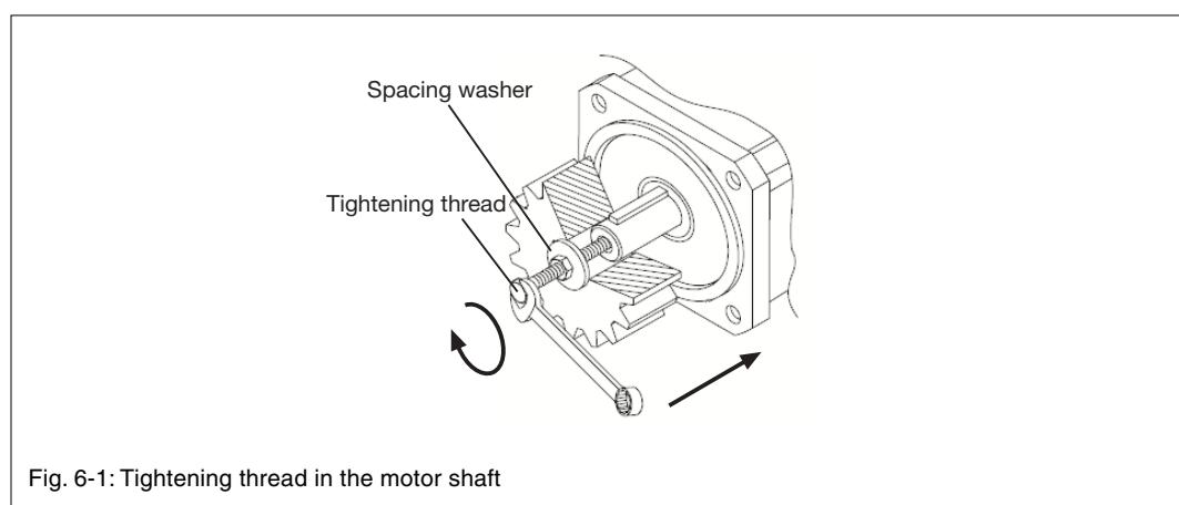
Fig. 6-1: Tightening thread in the motor shaft
