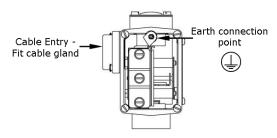
Figure 1: Parts location for wiring
