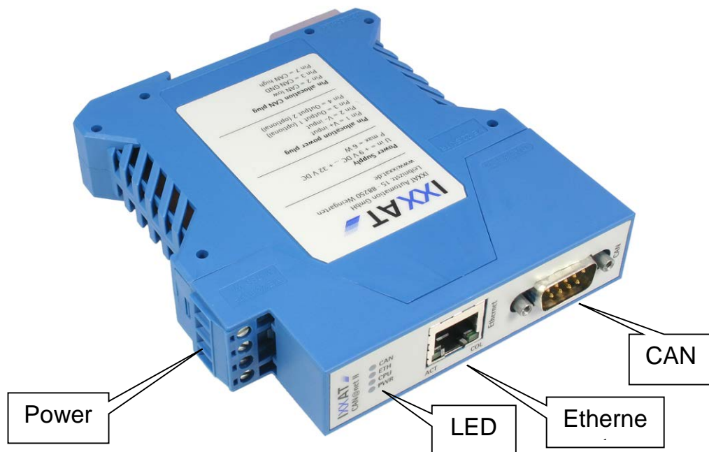
Figure 3-1 Connectors and displays of the CAN@net II/Generic
