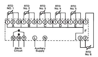
When used for less than 6 RTD inputs the unused terminals 1, 2 and 3 must be linked together.
