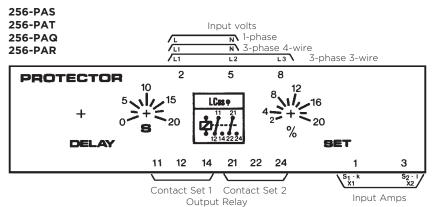
**Note:** Only one CT connection is required, from the same phase as the voltage connection to terminal 2.
