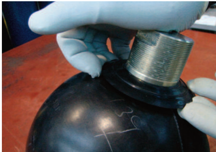
- Remove the gas valve, tilting slightly
