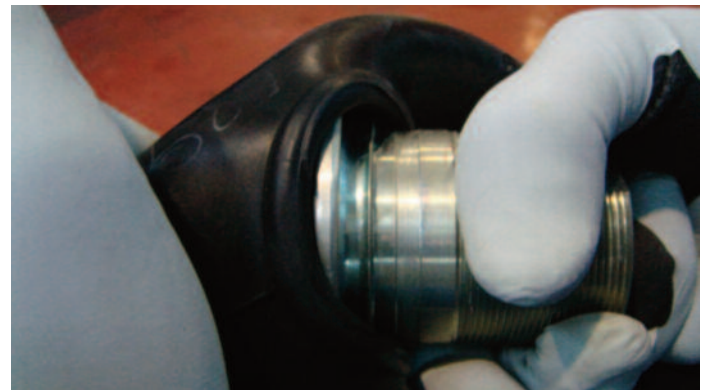
- Remove the gas valve, tilting slightly
