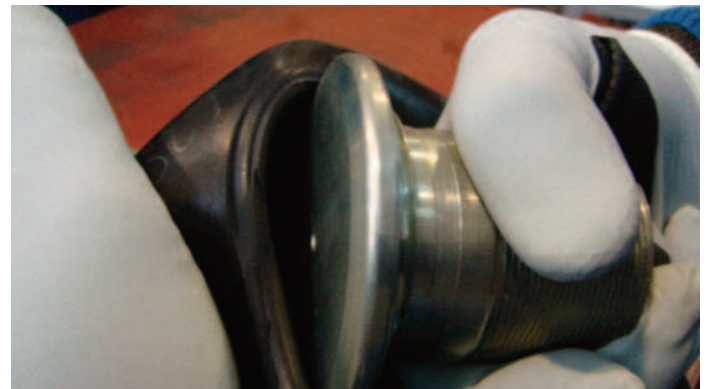
- Remove the gas valve, by pulling the bladder whit hand
