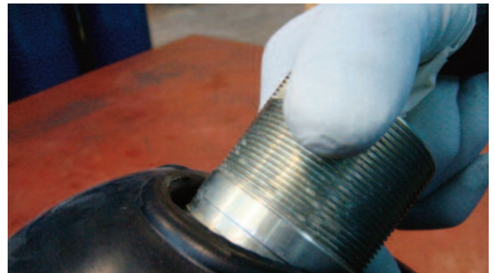
- Remove the gas valve, tilting slightly
