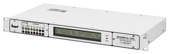
front view 8030HEPTA with at-a-glance status-LEDs and LCD Display
