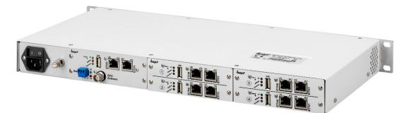
rear view base system 8030HEPTA extended with 4 mutually independent network time server modules 8030NTS/M
