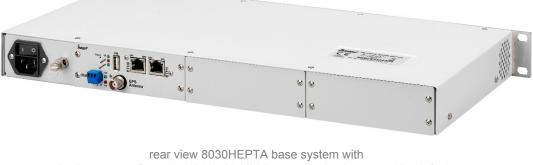
2 ethernet interfaces 10/100/1000 Mbit/s autosensing integrated by default, 1 USB-port and status LEDs
