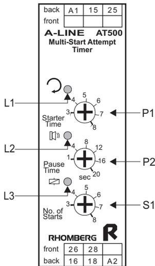
L1: The red “Starter” LED marked illuminates when the starter relay is energised.
