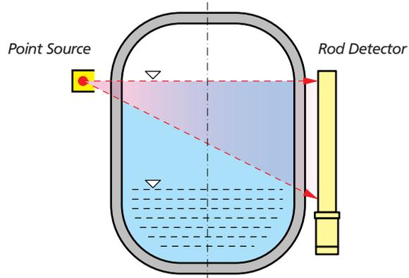
Figure 4: Rod Detector
